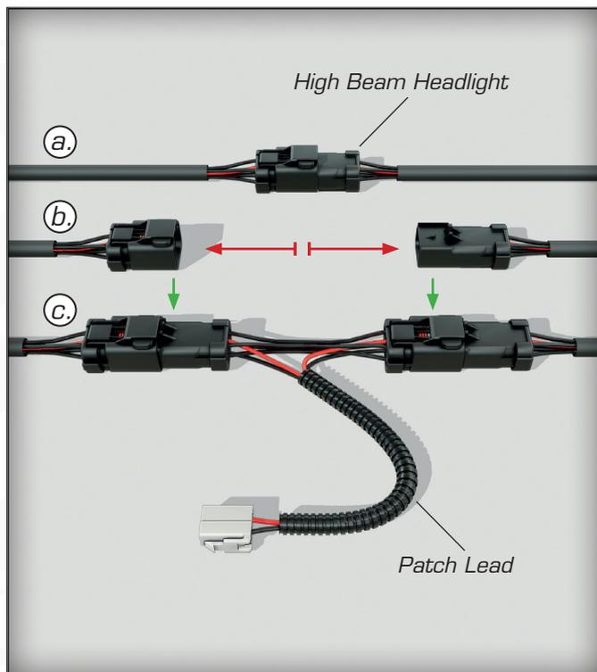
**2.** Disconnect High Beam Headlight plug & patch in supplied loom inline.
