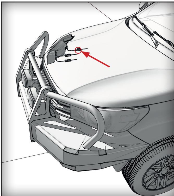
**1.** Locate High Beam Headlight plug in engine bay.
