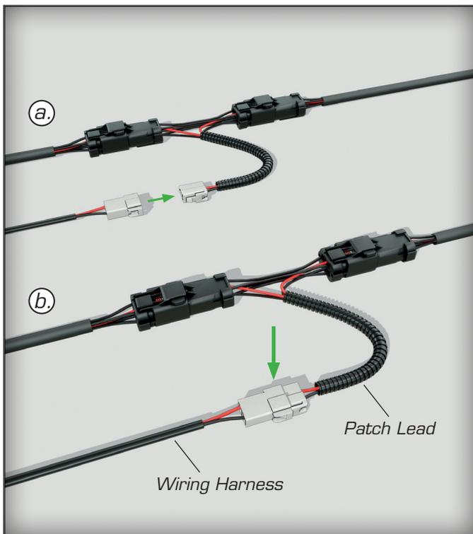
**3.** Complete connection by joining the Wiring Harness plug to Patch Lead plug.
