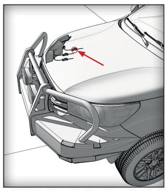
**1.** Locate High Beam Headlight plug in engine bay.
